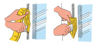
ISOVER Stopping Insulation is cut so that the wool overlaps with app. 15cm. Fig. d. All cuttings must be done in vertical joints. In prefabricated constructions with wodden elements ISOVER Stopping Insulation can be fixed on the elements before mounting.
